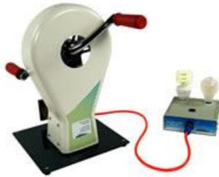
This demonstrates how much physical energy is required to produce enough power to light a 50 watt incandescent bulb versus a 15 watt CFL bulb.
