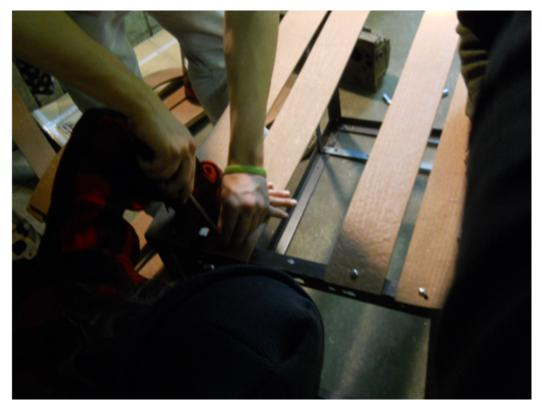
Team drilling holes through metal and screwing side pieces to bins.
