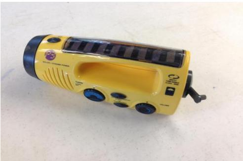
A fun way to explore PV with the option of a hand crank to compare the energy output.
