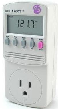
Have you ever wondered how much energy your lap top uses? Is a fan more energy efficient than an air conditioner? The Kill A Watt meter is a device that can help to answer these questions. Simply plug your appliance into the meter and plug the meter into the outlet. It will automatically record the amount of electricity used by the appliance. The electrical usage can also be converted to dollar value per day.
