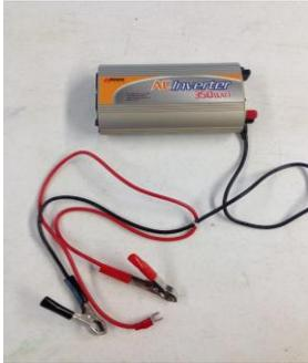
Most alternative energy systems create electricity in a Direct Current (DC) mode, but our appliances run on Alternating Current (AC). The use of an inverter will change the energy into a more useful form. The inverter can be used in conjunction with the PV panels or the Wind Turbine to assess how much energy these tools can actually produce.
