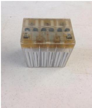
Students often wonder what a lead acid battery looks like inside. This model has a clear case so all the components are visible. There is no acid loaded in the battery, so it will not hold a charge.
