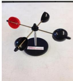
Four different models of anemometer that can be used to test wind speed at your school
